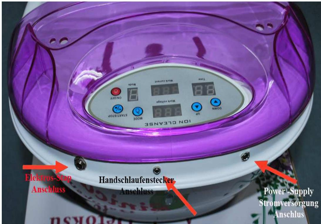
Elektro-Stap Anschluß = Electrical coil connection
